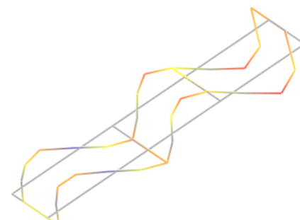
SelBand MIMO 2 : Mode 7 - Freq. 263.20Hz, Damp. 0.23%
